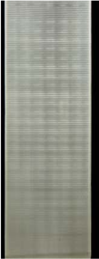
Figure 16. Enlarged image of 0.2mm FFF with uniform luminance. Dot size 30-50um.
