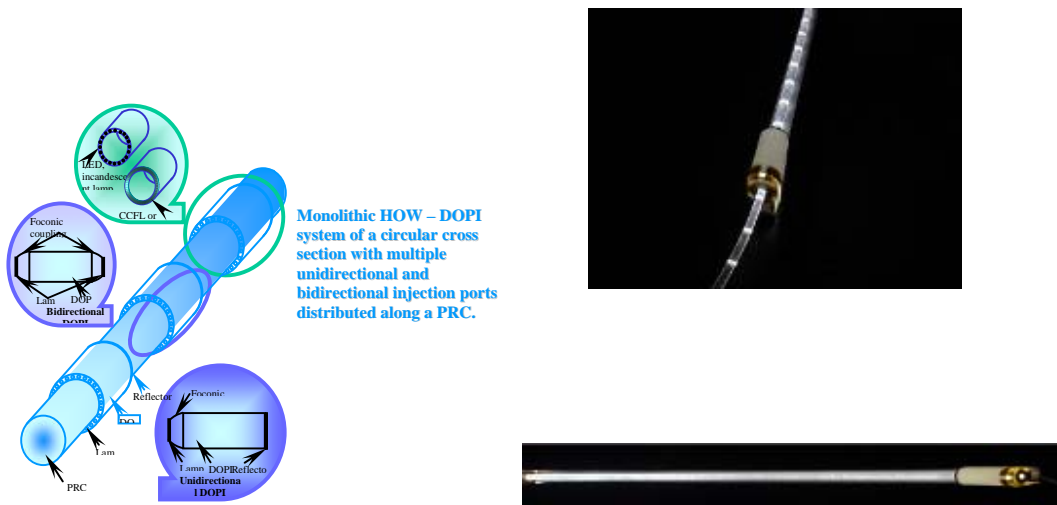
Figure 12. Doubly Hybrid PRC – DOPIs/DOPEs providing distributed flux injection and ejection over the whole length of PRC large core side emitting fiber for neon-like signage systems. This system enables to inject orders of magnitude higher flux into a core fiber and directionally ejects it without fiber attenuation losses, resulting in ground-breaking cost & performance improvements. Right: Actual devices with continuous & discrete lighting
