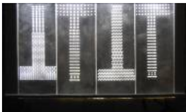
Figure 17. FFF with letter "T" for EXIT sign with directional microlens extractors.
